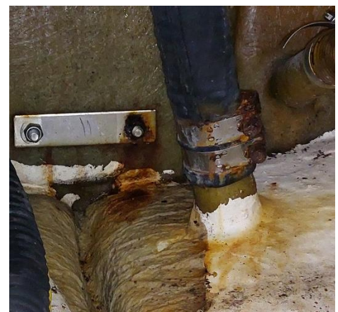
Check exhaust hose clamps.
