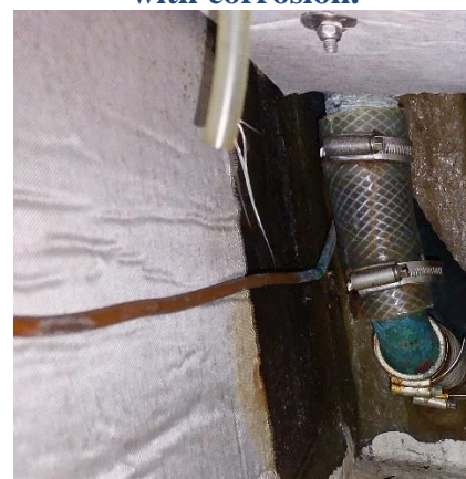
Corrosion and unsupported gas pipe under cockpit.
