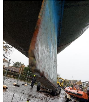
End of keels with damage noted.
