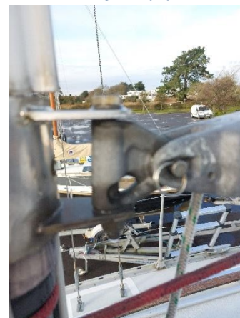
Attend to wear in gooseneck By fitting washers.
