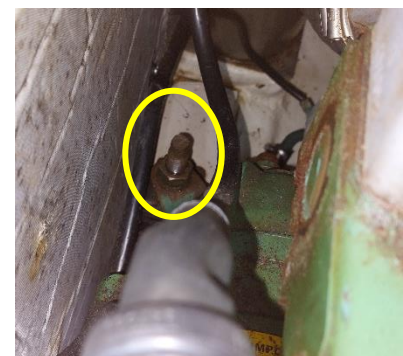
Attend to loose mount nut and further check engine mounts underload as considered soft.
