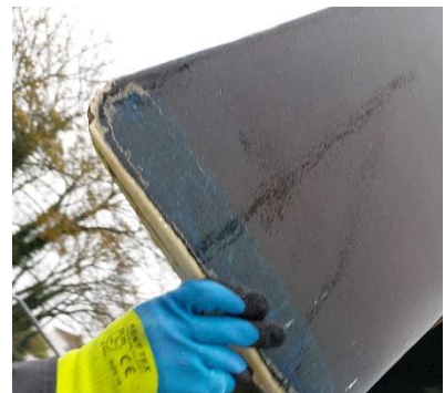
Rudder blade tip base damage.
