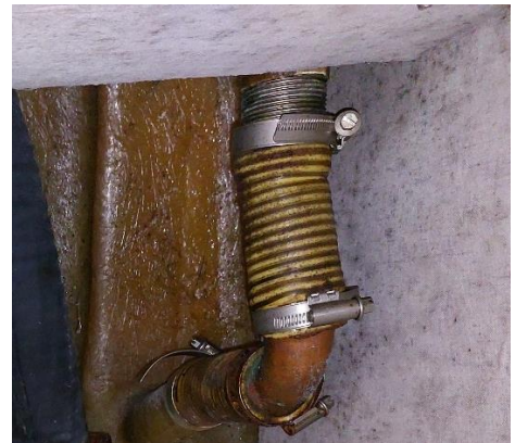
Cockpit hose drain as viewed may be in poor condition.
