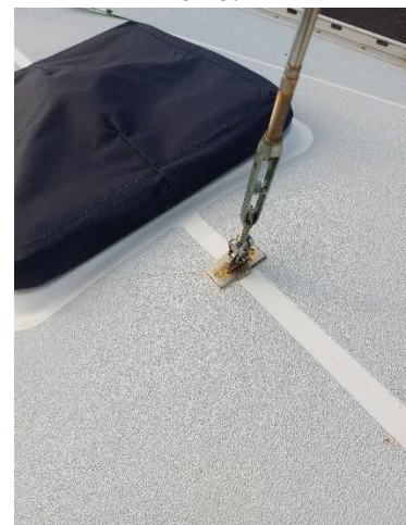
Attend to moisture ingress to baby stay and balsa core
