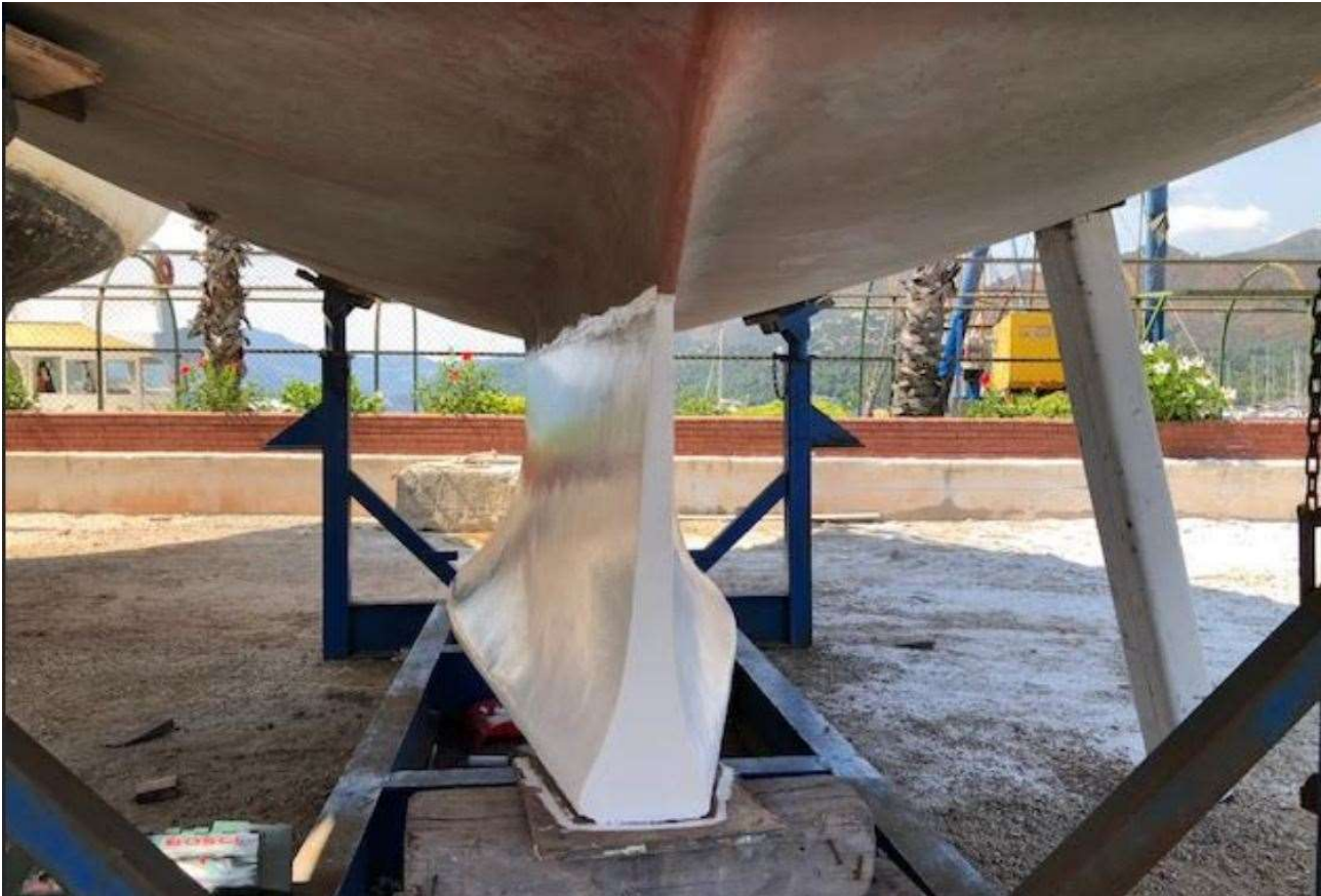
Scheel keel and old prop showing "stripper" rope cutter, shaft and hull anodes
